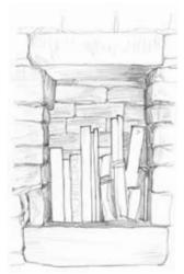
4 Reminiscent of traditional architecture, the recesses installed in a thick wall release small storage or simply decorative spaces and can enhance a less expressive stone wall.
